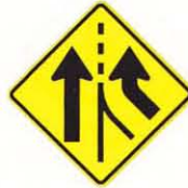
Added Lane Right S3030W43REA
